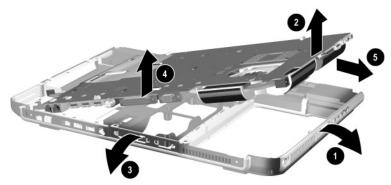
Removing the System Board
